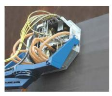
The blasting head seals directly onto the hull surface and is connected to the vacuum unit via a hose/pipework combination
